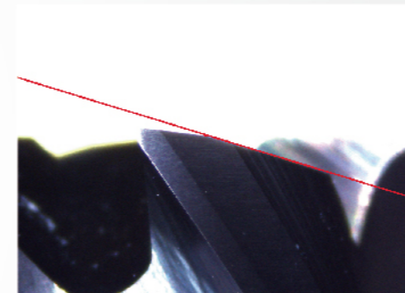
端刃第二後角 Second Rear Angle
